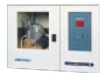
**Depolox® Basic Analyzer:** A low-cost analyzer for monitoring free or total chlorine residuals in drinking water applications. Provides a 4-20 mA output signal for recording or remote alarm devices. See TI 50.565 UA.
