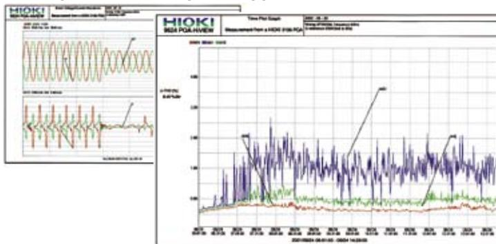
Print example: TIME PLOT screen (U-THD RMS fluctuation) printed on A4 paper
