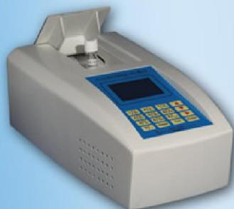
The ET1151M spectrophotometer is a microprocessor-controlled, LED-sourced filter photometer suitable for colorimetric testing in the laboratory or the field. The instrument is precalibrated for COD, TP and TN measurements and includes convenient calibration capability for user-entered methods.
